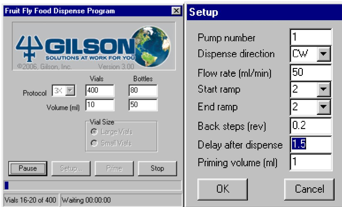
**Figure 8.** Software program for operating the automated 215 Fly Food Dispenser System with a Watson Marlow Pump.
