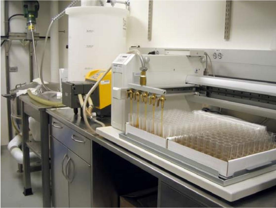
**Figure 6.** Typical layout of a fruit fly food dispensing system. Note that some of the plumbing fixtures/connections may vary. The system can be customized to suit the needs of the lab.
