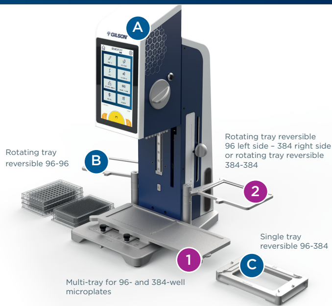
Figure 1 PIPETMAN® M96 accessories description
