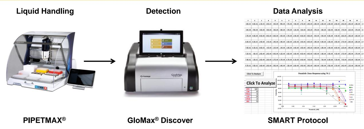
Figure 2. Reaction assembly, detection, and data analysis are automatically conducted according to user-input parameters for single or dose-response testing of up to two kinase strips per plate. Automated data analysis tools compute % kinase activity for up to twenty compounds (single-dose inhibition profile), or  $IC_{50}$  values for ten-point titration of up to two compounds (dose-response profile).
